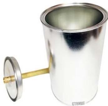
Stainless steel mortar boxes according to EN 196-9
